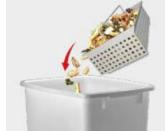
3. Empty the contents of the grease separator into a suitable container.
